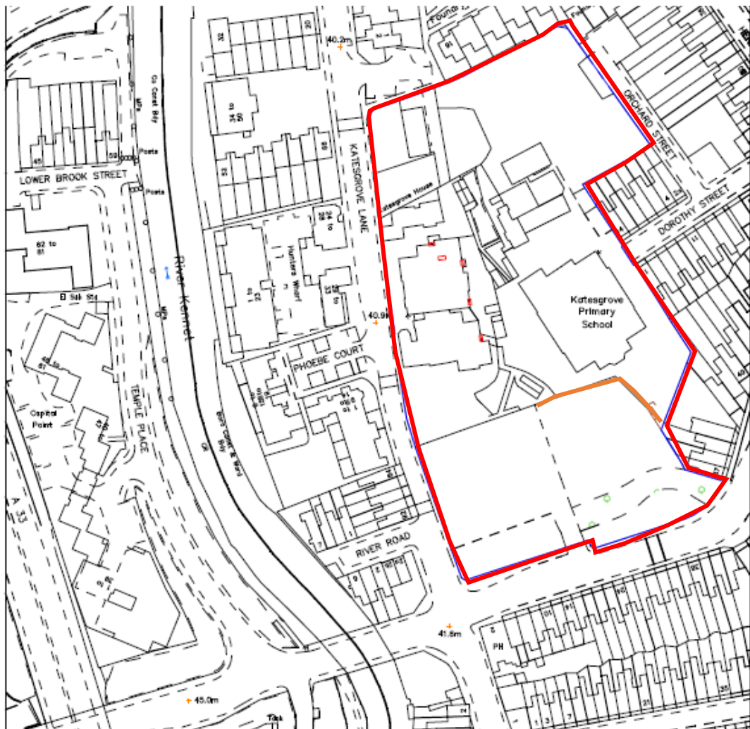
Red squares indicate flue works, orange line shows extent of buttress works
